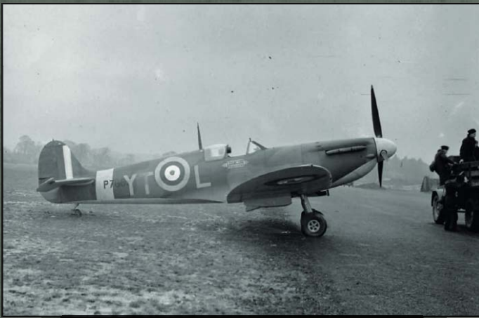
Spitfire Mk.IIa, P7665, of No. 65 Squadron at RAF Tangmere in the winter of 1941 (early 1941). Visible are the characteristics of the Spitfire Mk.IIa: the small bulge on the nose over the cartridge starter, the constant speed Rotol RX5/1 propeller with metal blades, the typical rounded spinner, antenna mast without a wire with insulator, antenna mast at the fin tip, IFF antennas spanning between the fuselage sides (note the grommet on the edge of the red and white segment of the fuselage roundel) and the leading edge of the horizontal stabilizer, and the standard rearview mirror. (photo: Simon Erland)
